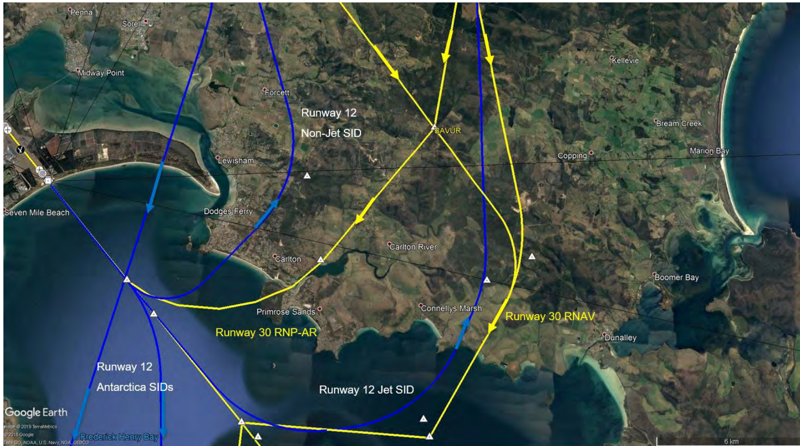
Figure 4 – Final Design (March 2019) - Zoomed in image showing Runway 12 departures and Runway 30 arrivals in the South East region; arrivals (yellow); departures (blue); waypoints (white triangles)
