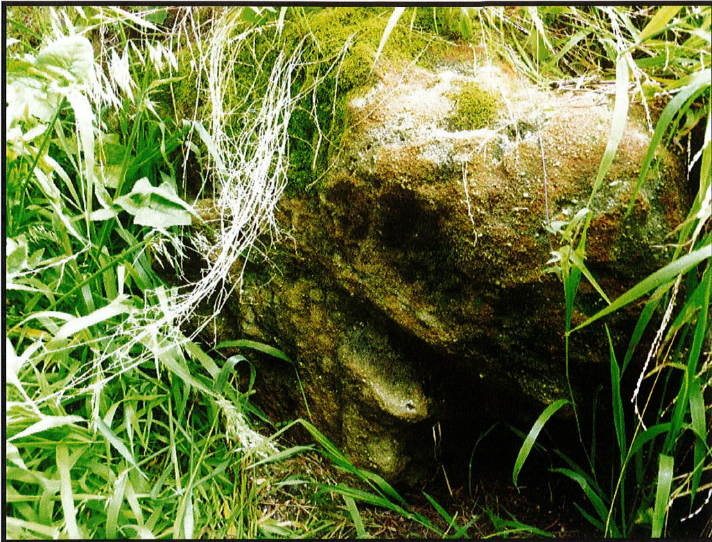
Photograph 17 – Photograph captured 13 October 2021. View of rock outcrop along the southern side of the subject land (i.e. long 1 Campbell Grove boundary). No evidence of loose / displaced soil at the toe of the rock outcrop.
