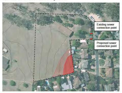
Figure 6-4 Sewer serviceability constraints for the existing sewer connection and proposed sewer connection
