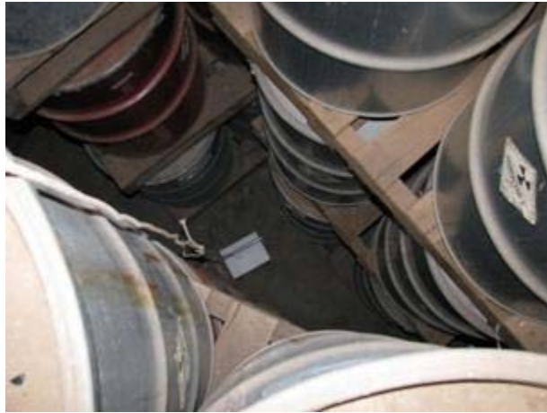
Photo 3: The SARAD radon monitor was lowered into a gap in the drums to measure the radon concentration at ground level.
