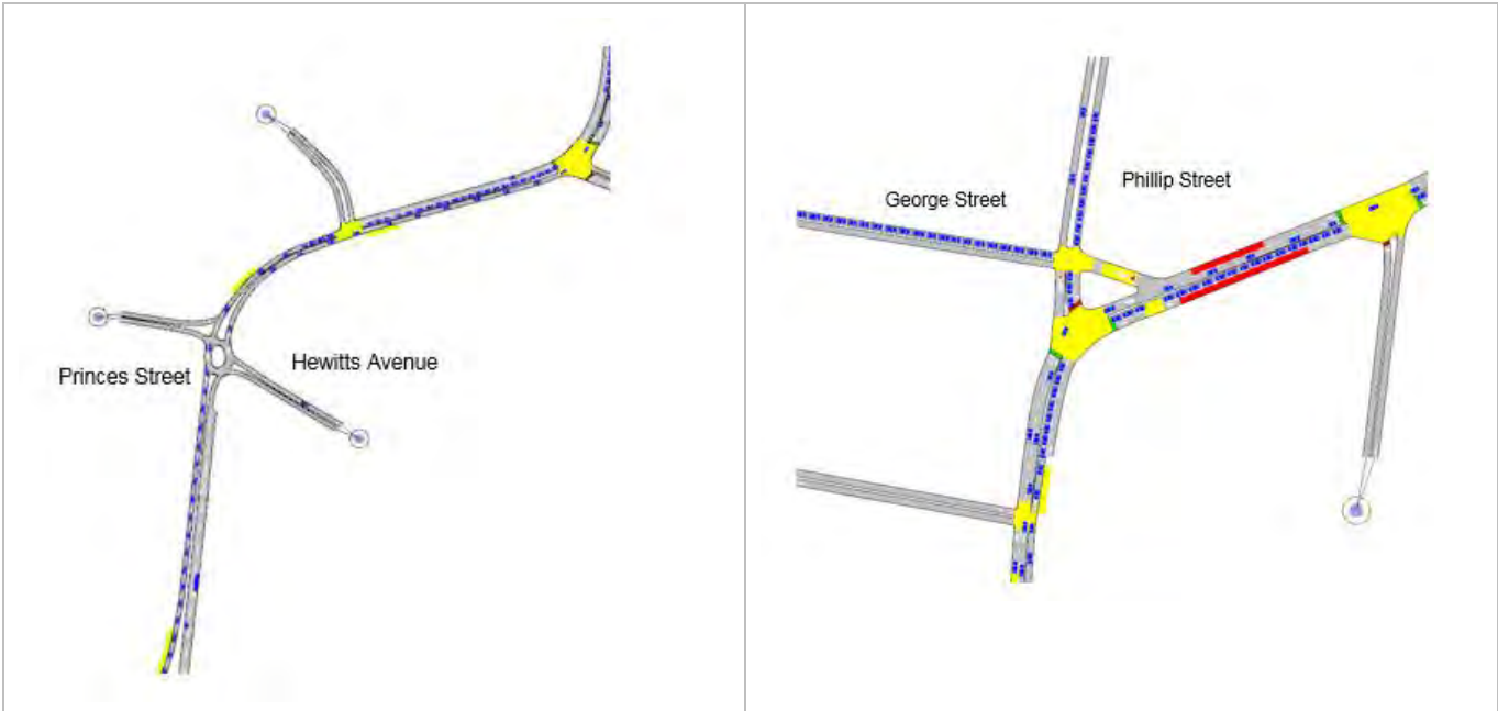
Northbound queuing on Lawrence Hargrave Drive extend back to south of Hewitts Avenue – PM peak 2026 and 2036
